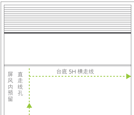
Cabling and Socket Under Work Surface with Vertical Internal Raceway
